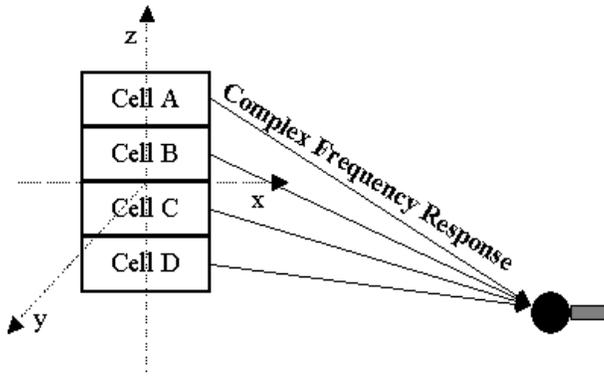
**Fig. 7. Using Superposition to Find the Response at Any Location**
