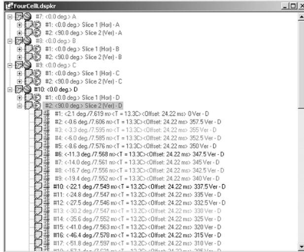
**Fig. 5. Tree View of a Simplified Loudspeaker Directional Response Object**
