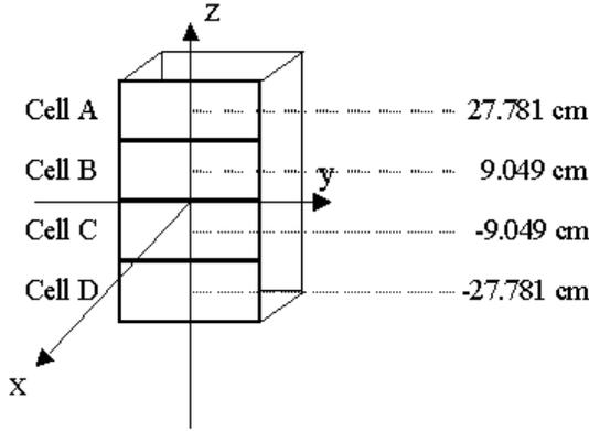
**Fig. 3. Loudspeaker Cell Locations**
