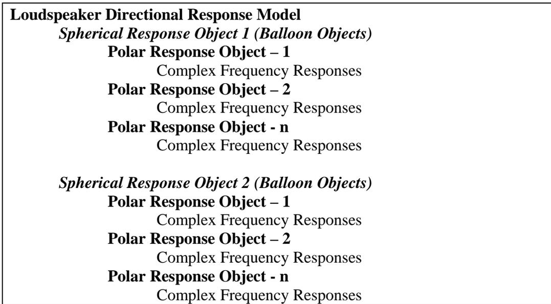
**Fig. 1. Loudspeaker Directional Response Model Hierarchy**
