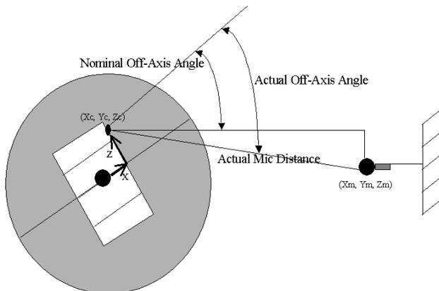
**Fig. 4. Calculating the Actual Microphone Angle and Distance**
