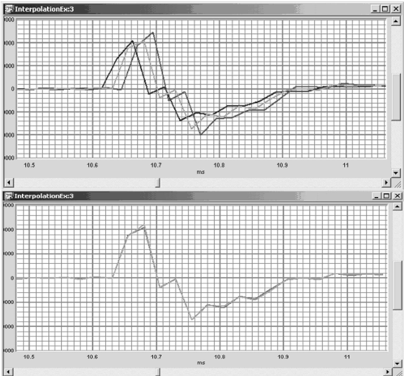
**Fig. 13. Interpolation Example: Time Domain. Top: Data measured at 10.7° and 16.0° with interpolated result at 13.4°. Bottom: Data measured and interpolated at 13.4°.**
