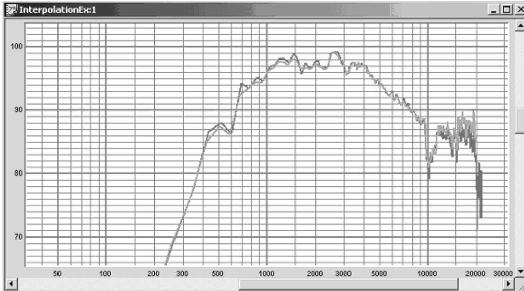
**Fig. 12. Interpolation Example: Magnitude. Top: Data measured at  $10.7^\circ$  and  $16.0^\circ$  with interpolated result at  $13.4^\circ$ . Bottom: Data measured and interpolated at  $13.4^\circ$ .**
