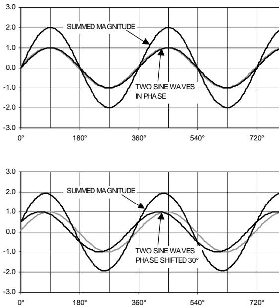
**Fig. 2. Sine wave magnitudes added in phase (top) and phase-shifted  $30^\circ$  (bottom)**
