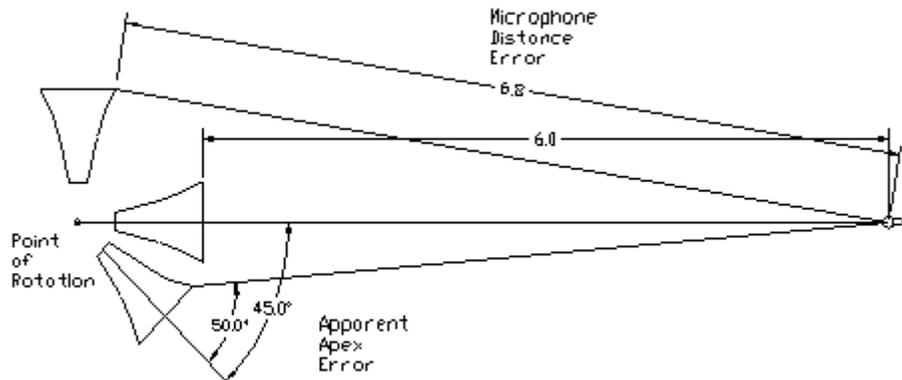
**Fig. 14. Apparent Apex Error**
