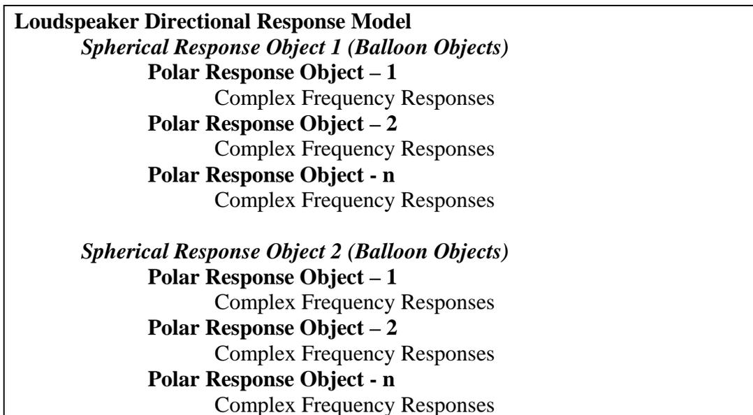
**Fig. 1. Loudspeaker Directional Response Model Hierarchy**
