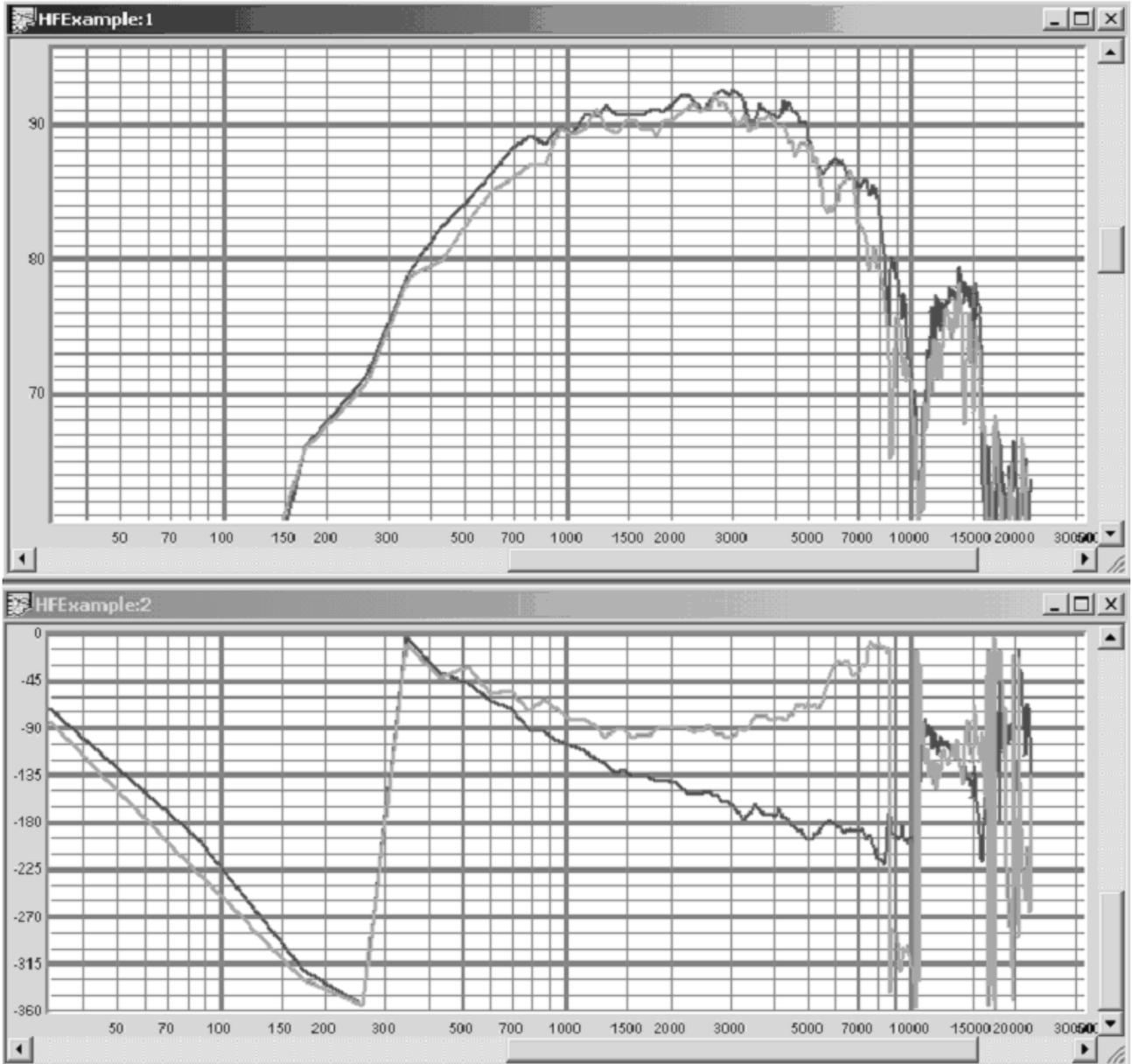
**Fig. 9. Two HF Transducers Measured Independently. Top: Magnitude. Bottom: Phase.**
