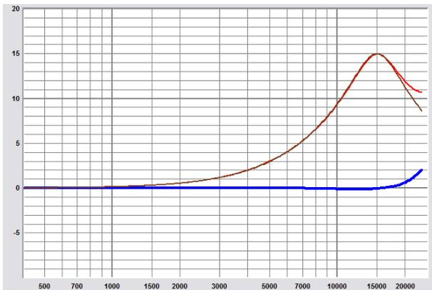
Figure 11: Biquadratic MZTi Bell Filter, 15 kHz, +15 dB,  $Q = 2.0$
