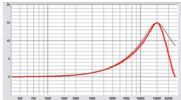
Figure 1: Analog vs. BZT Bell Filter, 15 kHz, +15 dB, Q = 2.0, SR = 48 kHz
