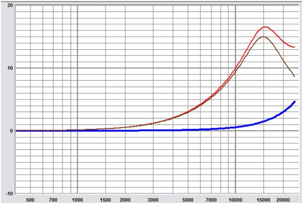
Figure 8: Error Function, Analog vs. MZT Response, 15 kHz Bell Filter (Q = 2.0)
