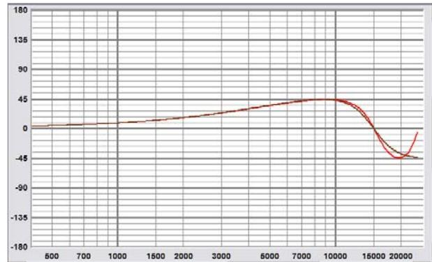
Figure 12: BZT Bell Filter Phase Response
