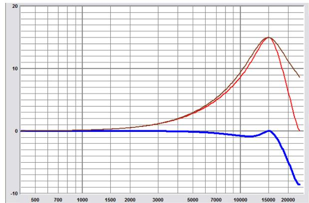
Figure 6: Error Function, BZT Bell Filter, 15 kHz, +15 dB,  $Q = 2.0$
