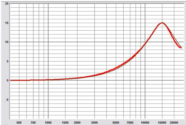
Figure 3: Analog vs. Orfanidis BZT Bell Filter, with pre-warped  $f_2$
