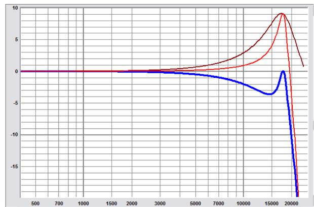
Figure 5: Error Function, BZT Low-pass Filter, 18 kHz,  $Q=2.8$
