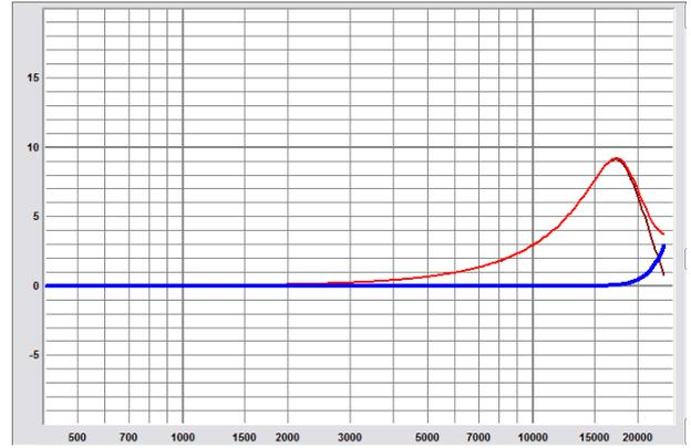
Figure 9: MZTi Low-pass Filter, Single-Zero Correction Filter, 18 kHz, Q = 2.8
