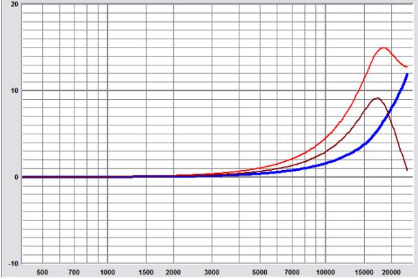
Figure 7: Error Function, MZT Low-pass Filter, 18 kHz, Q=2.8
