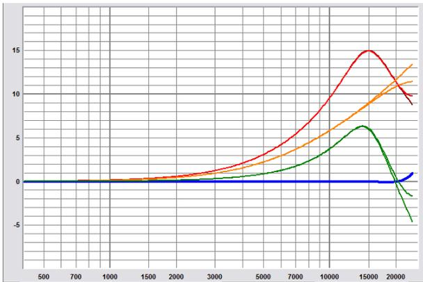
Figure 10: Bicubic MZTi Bell Filter And Partial Filters, 15 kHz, +15 dB, Q = 2.0
