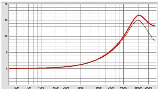
Figure 4: Analog vs. Standard MZT Bell Filter, 15 kHz, +15 dB,  $Q = 2.0$
