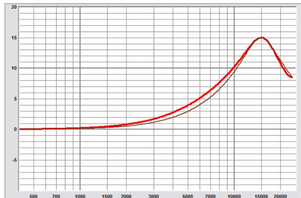
Figure 2: Analog vs. Orfanidis BZT Bell Filter, 15 kHz, +15 dB, Q = 2.0, SR = 48 kHz
